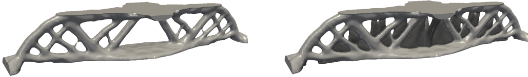
Figure 7: Test Case 5 (3D beam): fixed shape (left) and its optimal support (right).
