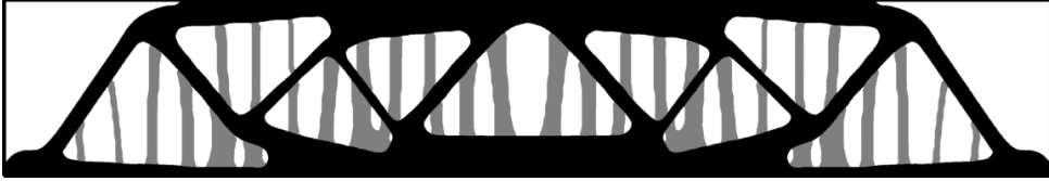
Figure 11: Test Case 9: Optimal supports with respect to the average of mechanical and thermal compliances.
