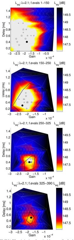
Fig. 8. UH-CMA-ES optimization of a gain-delay controller for  $\lambda = 2.1$ , heating up. Function evaluations, from top plot down: 1–150; 150–250; 250–325; 325–390. Pentagrams show the best parameter set for each generation, the larger they are, the later they have been acquired for each plot. The black polygon is the convex hull of all controller parameter values tried in the given time range.
