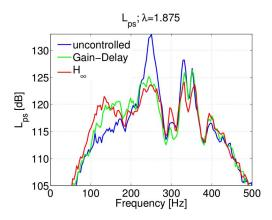
Fig. 14. Comparison of the pressure spectra when the plant is uncontrolled, gain-delay and  $\mathcal{H}_{\infty}$  controlled. Both controllers are UH-CMA-ES optimized,  $\lambda = 1.875$ .
