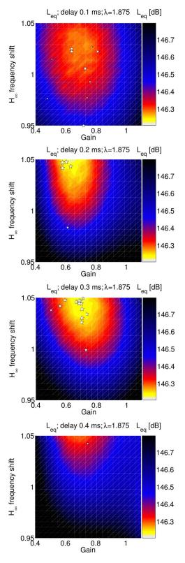
Fig. 12. UH-CMA-ES optimization of an  $\mathcal{H}_{\infty}$  controller for  $\lambda = 1.875$ . Delays from top plot down: 0.1–0.4 ms. Pentagrams show the best parameter set for each generation.
