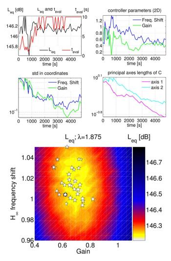
Fig. 10. Parameter evolution for the UH-CMA-ES optimization of a  $\mathcal{H}_{\infty}$  controller for  $\lambda = 1.875$  (top) and the resulting cost function landscape (bottom). Pentagrams show the best parameter set for each generation.
