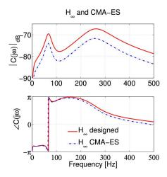
Fig. 16. Designed and UH-CMA-ES-optimized  $\mathcal{H}_{\infty}$  controller for  $\lambda = 2.1$ .
