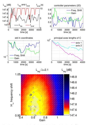
Fig. 15. Parameter evolution for the UH-CMA-ES optimization of an  $\mathcal{H}_{\infty}$  controller for  $\lambda = 2.1$  (top) and resulting cost function landscape (bottom). Pentagrams show the best parameter set for each generation.
