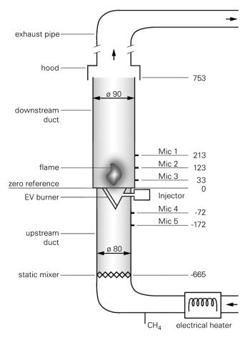
Fig. 1. Illustration of the ETH combustor. Preheated air premixed with methane enters the upstream duct, the flame is stabilized by the EV burner. All dimensions in millimeters.
