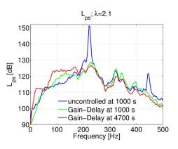
Fig. 6. Comparison of the uncontrolled and controlled spectra of the pressure signal at 1000 s and 4700 s for the same gain-delay controller and  $\lambda = 2.1$ .
