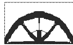
Fig. 9. Bridge arch resulting from penalizing the composites from the start of the algorithm
