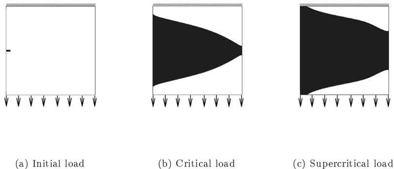
Figure 1: Mode  $I$  damage for the  $320 \times 320$  mesh with 100 time steps. Initial configuration with an imposed displacement of 0.02 (a) critical load at an imposed displacement of 0.006 (b) and supercritical load with an imposed displacement of 0.072 (c).
