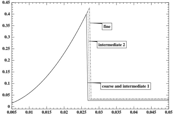
Figure 8: Third mesh convergence test for the mode  $I$  crack: cost function (2.10) with respect to simultaneous mesh, crack and  $\kappa$  refinements for 100 time steps.
