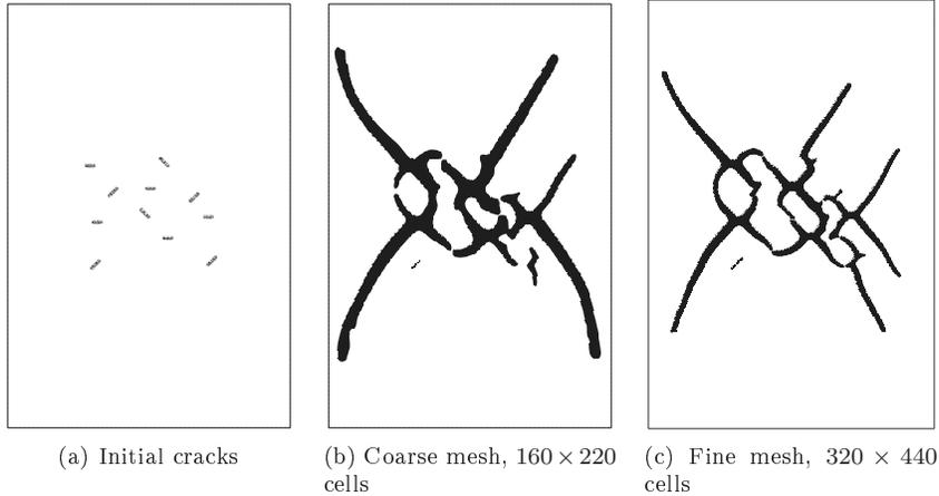
Figure 12: Multiple crack experiment with a mode II loading.
