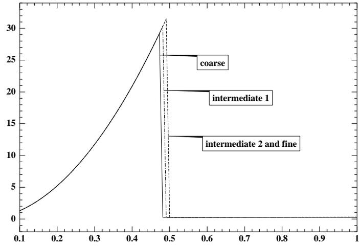
Figure 10: Mode II crack test: cost function (2.10) with respect to simultaneous mesh, crack and  $\kappa$  refinements for 100 time steps.
