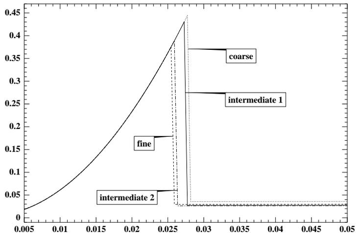
Figure 6: First mesh convergence test for the mode  $I$  crack: cost function with respect to the imposed displacement for various meshes and with 100 time steps.
