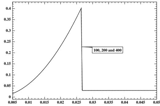
Figure 5: Time-step refinement for the mode  $I$  crack: cost function with respect to the imposed displacement for three time refinements.
