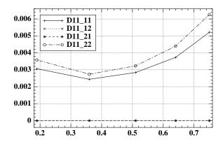
Figure 11: Electrodiffusion tensor  $\mathbb{D}_{11}$  for the cation versus porosity  $(n_j^0(\infty)=0.1 mole/l)$
