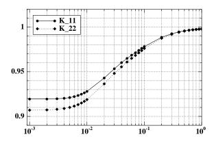
Figure 4: Diagonal entries of the relative permeability tensor,  $\mathbb{K}_{11}$  and  $\mathbb{K}_{22}$ , as functions of the dimensional (mole/l) infinite dilution concentrations  $n_j^0(\infty)$
