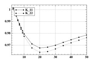
Figure 9: Relative permeability coefficients  $\mathbb{K}_{11}$  and  $\mathbb{K}_{22}$  versus pore size  $\ell$  (nm)
