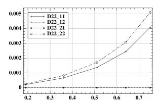
Figure 12: Electrodiffusion tensor  $\mathbb{D}_{22}$  for the anion versus porosity  $(n_j^0(\infty) = 0.1 mole/l)$
