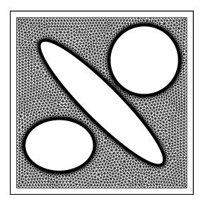
Figure 1: Mesh for a periodicity cell with ellipsoidal inclusions
