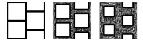
Figure 2: Meshes for three different porosities (0.19, 0.51 and 0.75) of a periodic cell with rectangular inclusions
