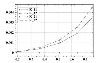
Figure 10: Permeability tensor  $\mathbb{K}$  versus porosity  $(n_j^0(\infty) = 0.1 mole/l)$
