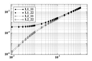
Figure 8: Diagonal entries of the coupling tensors  $\mathbb{L}_1$  and  $\mathbb{L}_2$ , as functions of the dimensional (mole/l) infinite dilution concentrations  $n_j^0(\infty)$  (log-log plot)
