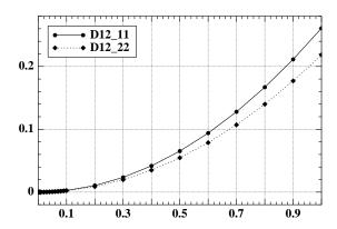
Figure 6: Diagonal entries of the cross-diffusion tensor  $\mathbb{D}_{12}$ , as functions of the dimensional (mole/l) infinite dilution concentrations  $n_j^0(\infty)$
