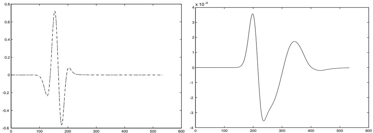
Figure 4: Pressure field (left) and error on the pressure (right) near the upperleft corner for a horizontal flow  $M = 0.33$  vs. time steps
