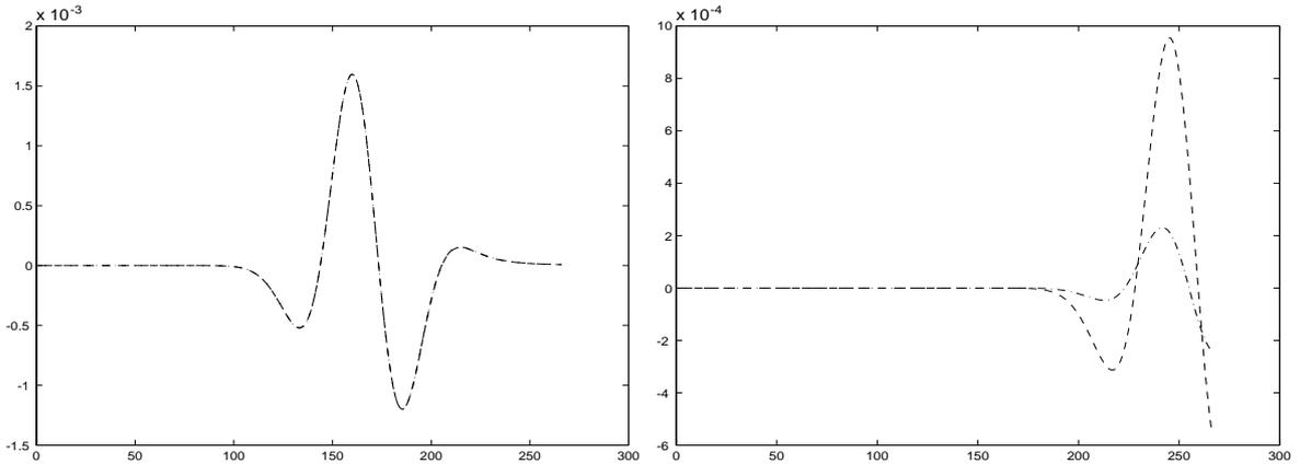
Figure 1: Pressure fields for the reference solution and the PML solution near the upperleft corner (left) and in the PML (right) for an oblique flow  $M = 0.33$  vs. time steps
