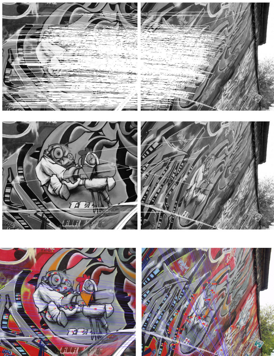
Figure 30: Correspondences between the images Graffiti 1 and Graffiti 6. Transition tilt: \tau \approx 3.2 . Top: A-SIFT finds 724 correspondences, out of which 3 are false. Middle: SIFT finds 6 correspondences. Bottom: MSER finds 127 correspondences, out of which 50 are correct. In this example, MSER is successful. But MSER fails to work under big image zoom or if the shapes in the images are not well contrasted.
