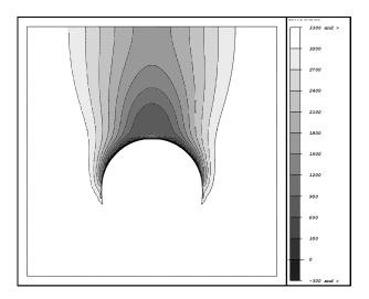
Figure 14: Fiber-reinforced matrix: isovalues of the topological derivative at the initialization.
