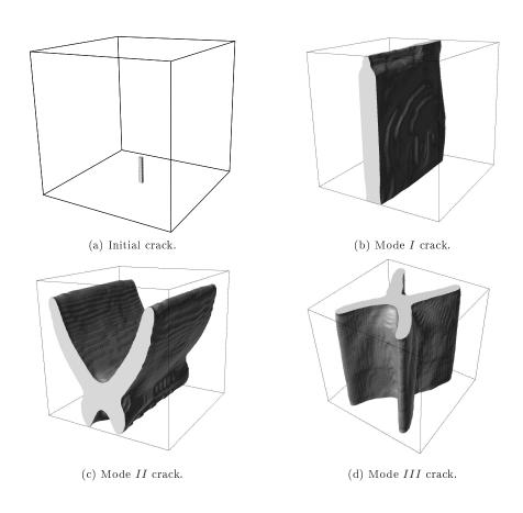
Figure 16: Initial and final cracks for the modes I,II and III in 3d.
