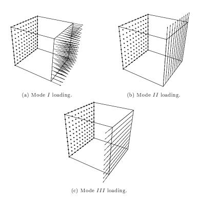
Figure 15: Boundary conditions for the modes I, II and III in 3d.
