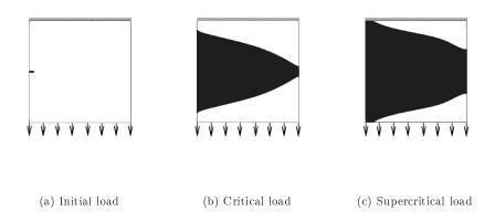
Figure 1: Mode I damage for the  $320\times320$  mesh with 100 time steps. Initial configuration with an imposed displacement of 0.02 (a) critical load at an imposed displacement of 0.006 (b) and supercritical load with an imposed displacement of 0.072 (c).
