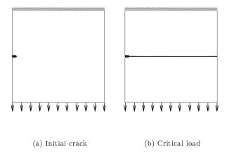
Figure 4: Mode I crack: initial configuration (a) and critical load at 0.0028 (b).
