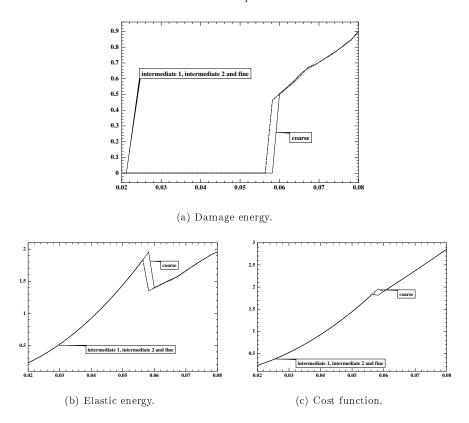
Figure 2: Mode I damage experiment: variations of various energies as functions of the imposed displacement. Griffith energy (a), elastic energy (b) and cost function (c) for four different mesh refinements with 100 time steps.
