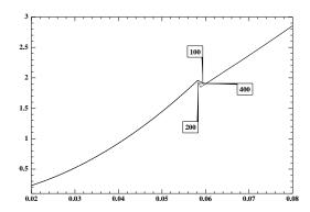
Figure 3: Mode I damage experiment: cost function with respect to the imposed displacement for the  $320 \times 320$  mesh and for 100,200 and 400 time steps.
