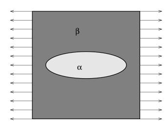
Let  $D = ]0; 1[\times]0; L[$  be a rectangle in  $\mathbb{R}^2$ . We fill D with a mixture of two materials, homogeneous isotropic, characterized by an elasticity coefficient  $\beta$  for the strong material, and  $\alpha$  for the weak material (almost like void) with  $\beta >> \alpha > 0$ . We denote by  $\chi(x) = 0, 1$  the **characteristic function** of the weak phase  $\alpha$ , and we define
