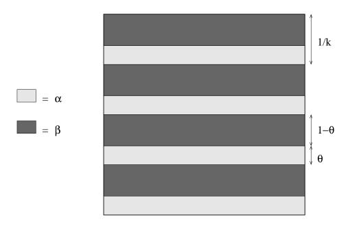
Minimizing sequence  $k \to +\infty$ : k rigid fibers, aligned in the principal stress  $e_1$ , and uniformly distributed. To achieve a uniform boundary condition, the fibers must be finer and finer and alternate more and more weak and strong ones.
