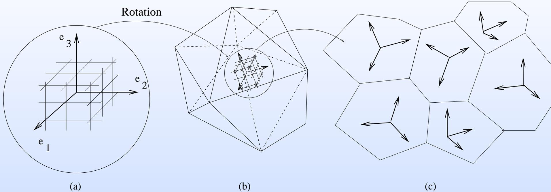
Each grain is a copy of the same single crystal, except for its orientation  $\theta$  which varies from grain to grain.
