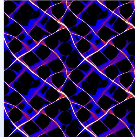
“Weak” configuration. More regular spatial arrangement. Shear bands running at  $\pm 45^0$  with respect to the tensile direction.
