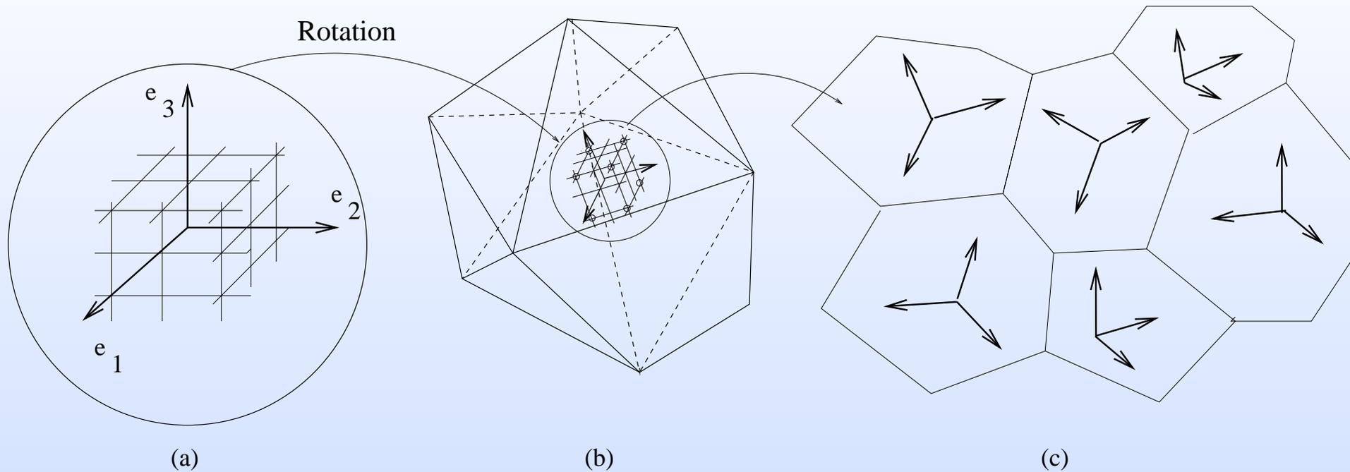
Each grain is a copy of the same single crystal, with energy  $w^s$  except for its orientation  $\theta$  which varies from grain to grain.
