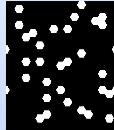
Covering by identical hexagons. Properties of the hexagons chosen randomly (phase 1 or phase 2). 200 different configurations for each volume fraction.
