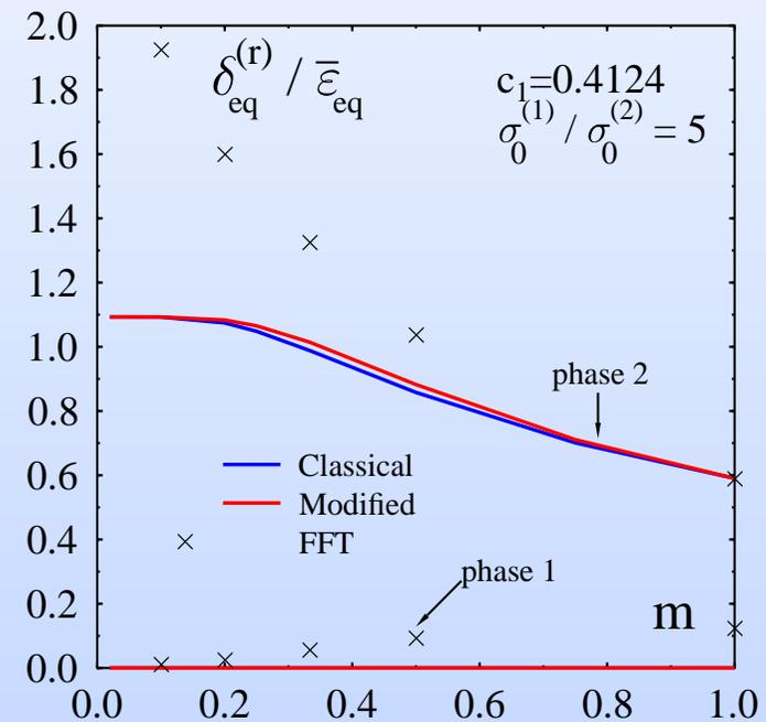
**Fluctuations of the strain in the matrix**  $\nearrow$  when  $m \searrow 0$ . Blow-up not well captured by the secant theories.
