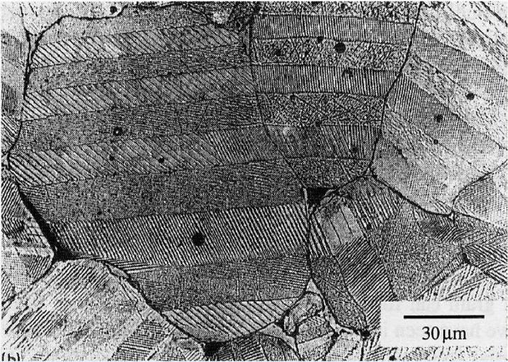
**Strain compatibility from one grain to another : strong geometrical constraint.**
