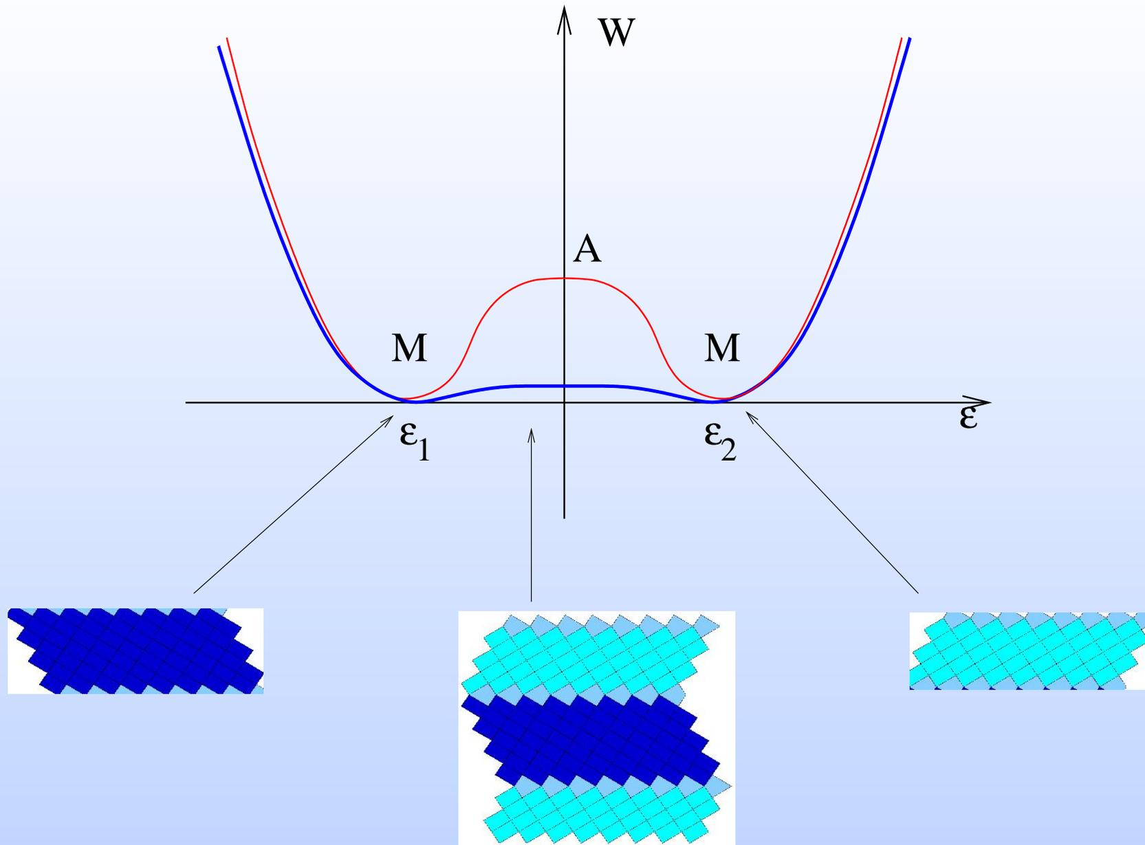
Note that there is a domain of **low energy** in strain space : **domain of recoverable strains for the single crystal.**
