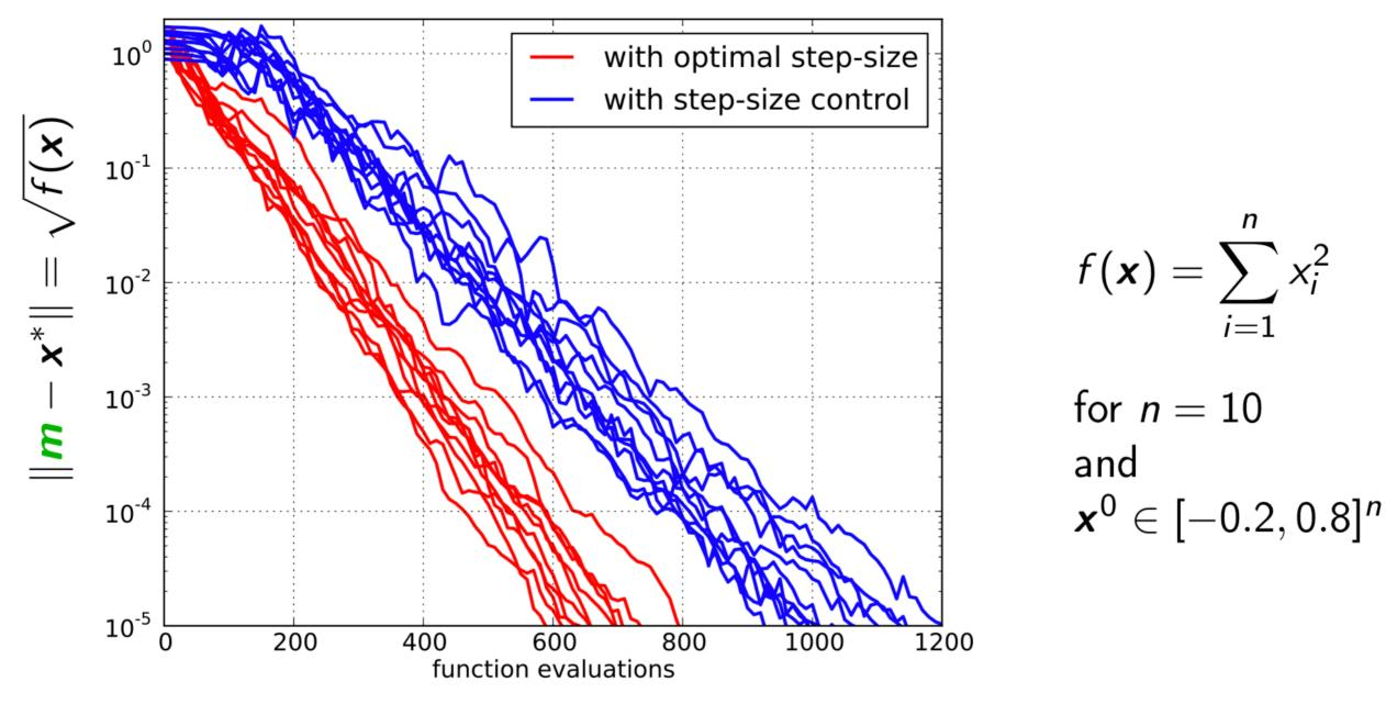
with optimal versus adaptive step-size  $\sigma$  with too small initial  $\sigma$
