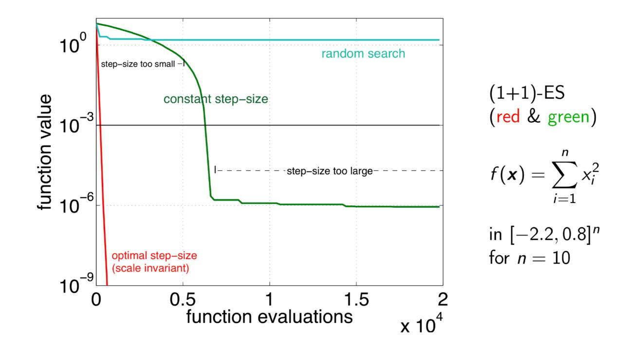
red curve: (1+1)-ES with optimal step-size (see later) green curve: (1+1)-ES with constant step-size ( $\sigma = 10^{-3}$ )
