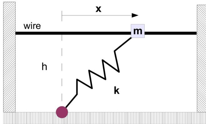
A bead of mass  $m$  is constrained to slide along a straight horizontal wire. A spring of relaxed length  $L$  and spring constant  $k$  is attached to the mass and to a support point at distance  $h$  from the wire. We suppose that the motion of the bead is opposed by a viscous damping force proportional to the speed with a factor  $b > 0$ .
