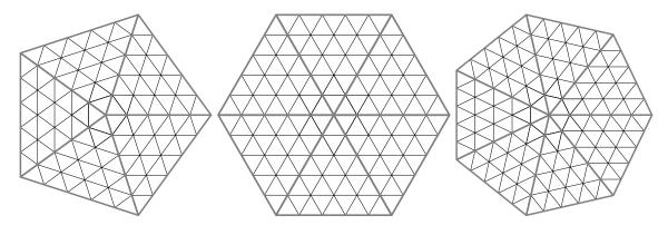
FIGURE 4. Examples of symmetric meshes for regular polygons used in the computations.
