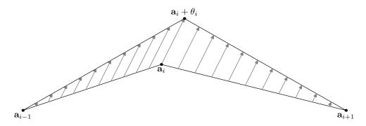
FIGURE 2. Boundary perturbation induced when perturbing a vertex
