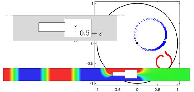
Figure 2: Zero transmission in a waveguide.
