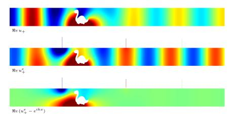
▶ Working a bit more, one can show that two resonators are enough to cloak any object.
