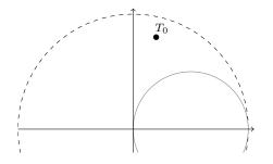
**Step 1**: add one ligament so that the corresponding transmission circle, which passes through zero and  $T_0$ , crosses  $\mathscr{C}(1/2, 1/2) \setminus \{0\}$ .
