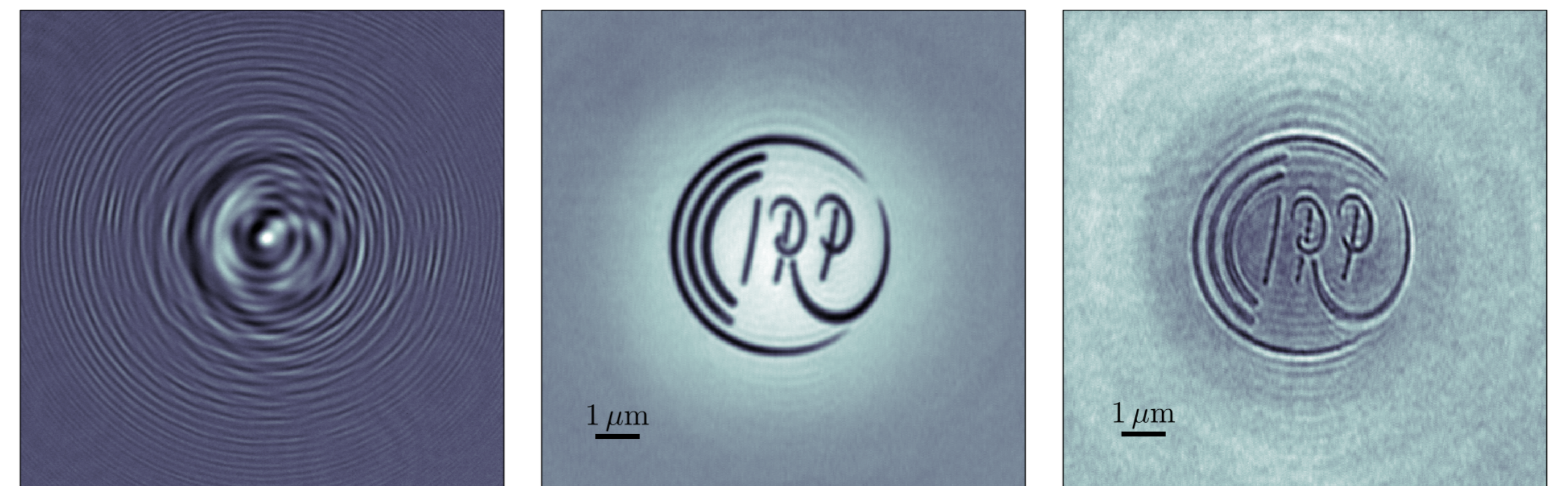
(a) Intensity data (GINIX/DESY [3]) (b) Reconstructed refraction \int_{-L}^0 \delta dz (c) Reconstructed absorption \int_0^d \beta dz
