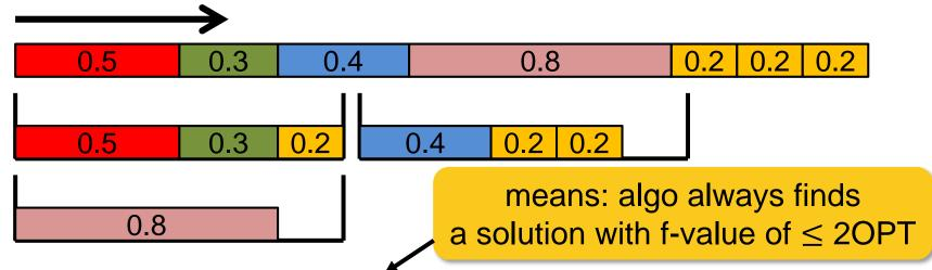
Theorem: First-Fit algorithm is a 2-approximation algorithm
