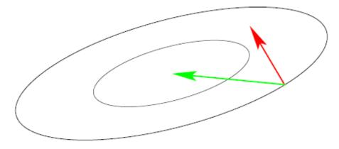
gradient direction  $-f'(x)^T$ Newton direction  $-H^{-1}f'(x)^T$
