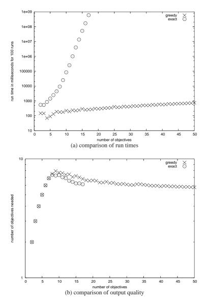
**Fig. 6.** Comparison between the greedy and the exact algorithm for the random problem and 32 solutions. Note that the plot of the running times in a) is a logscale plot and only the summed running times over 100 runs on a linux computer (SunFireV60x with 3060 MHz) are shown. Figure b) shows the sizes of the computed minimum / minimal sets averaged over 100 runs.
