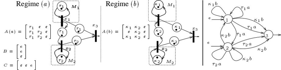
**Fig. 3.** A Workshop with Two Production Regimes and its Equivalent  $(\max, +)$  Automaton
