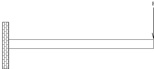
Figure 2: A cantilever beam with constant force F.
