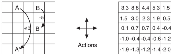
Figure 3.2: Gridworld example: exceptional reward dynamics (left) and state-value function for the equiprobable random policy (right).
