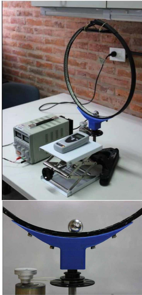
Figure 5. Experimental device. The smartphone used to record the motion can be seen at the top of the hoop.
