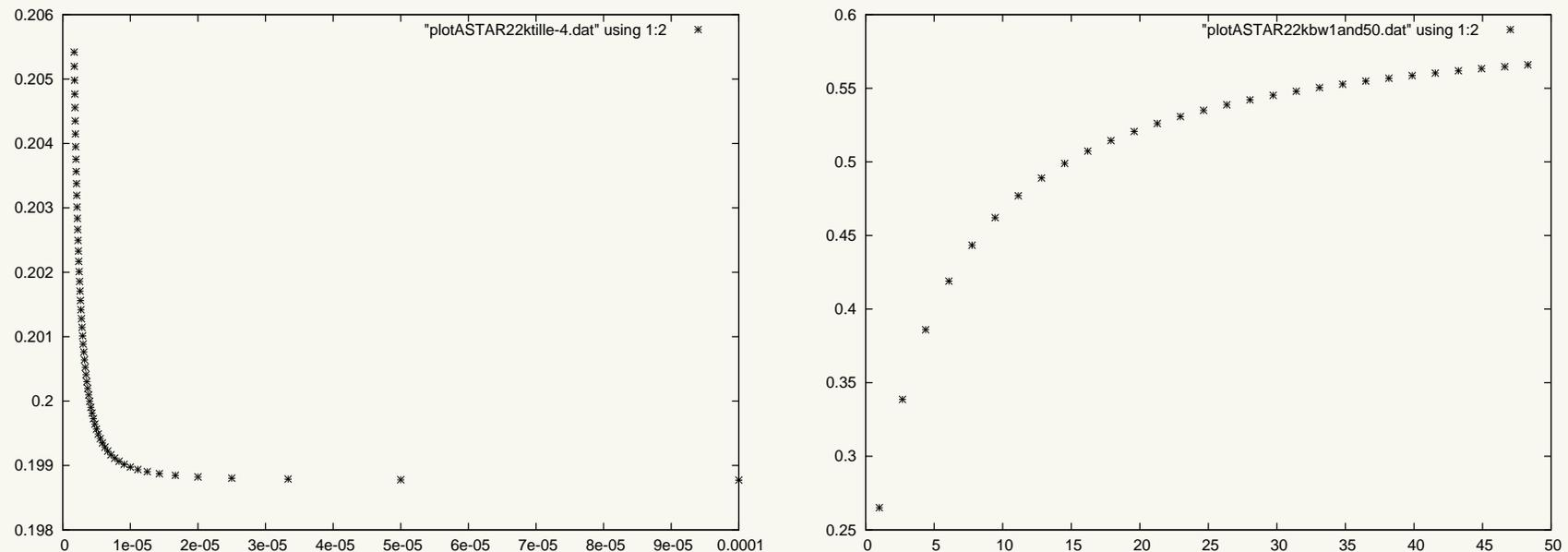
Figure 4: The variation of effective transverse diffusion: Left,  $\kappa$  tending to 0; Right,  $\kappa$  increasing in magnitude
