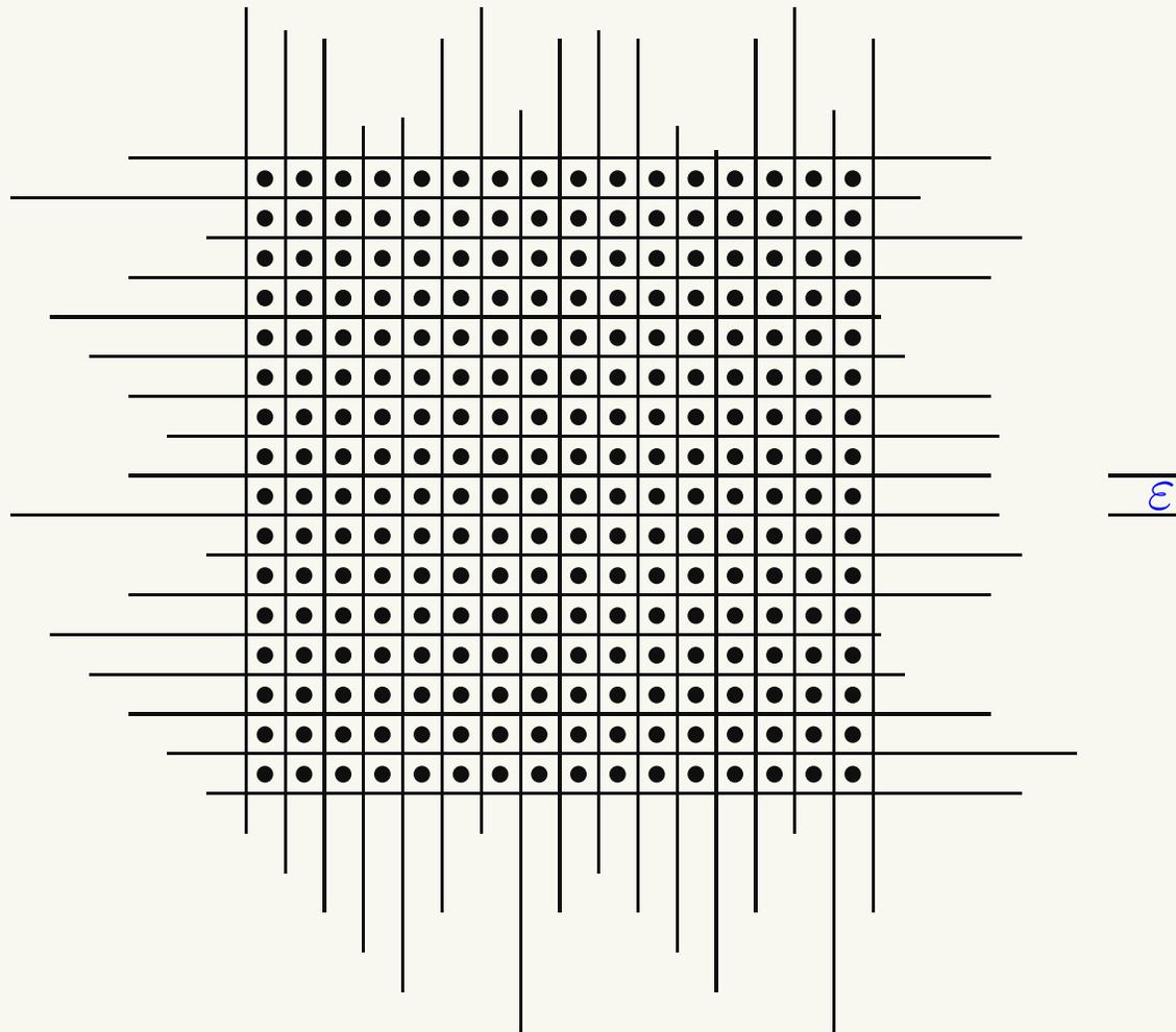
2-D schematic of an unbounded porous media
