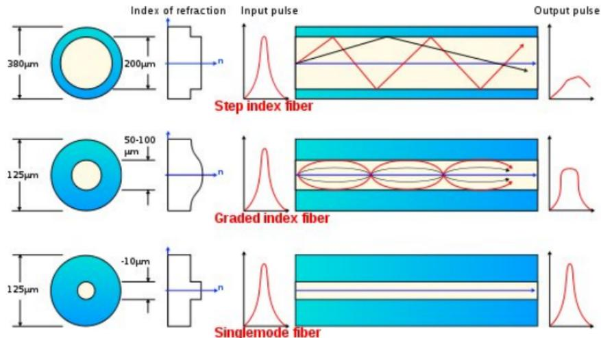
Core diameter may be less than 10 times the wavelength of the propagation light
