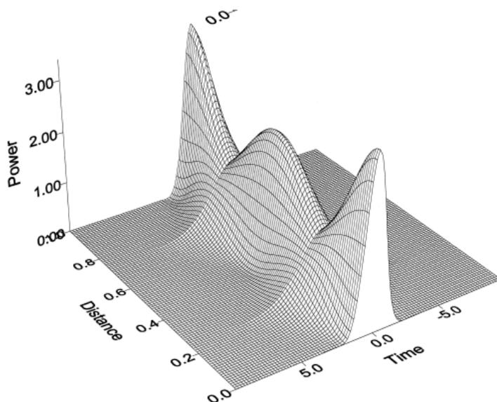
Fig. 1. Evolution over one compensation period of DM soliton shown in normal (bottom) and logarithmic (upper picture) scales. In the leading order the dynamics is self-similar (bottom) and is given by Eqs. (37). It is seen that the dips appear at the beginning (end) and in the middle of the periodic cell. Dispersion map  $d(z) = \bar{d} + \langle d \rangle = \pm 5 + 0.15$ ,  $c(z) = 1$ .
