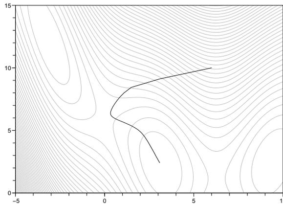
**Figure 14.7.** Example of a *steepdesc* execution with 100 iterations on the Branin-Hoo function.
