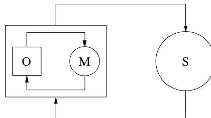
**Figure 14.3.** Example of an optimization procedure based on a metamodel. The group made of an optimizer and a metamodel yields a new optimizer which is coupled to a computationally expensive simulator. After each new simulation, the metamodel is updated. The solution point found by optimizing the metamodel is presented to the simulator at each outerloop iteration.
