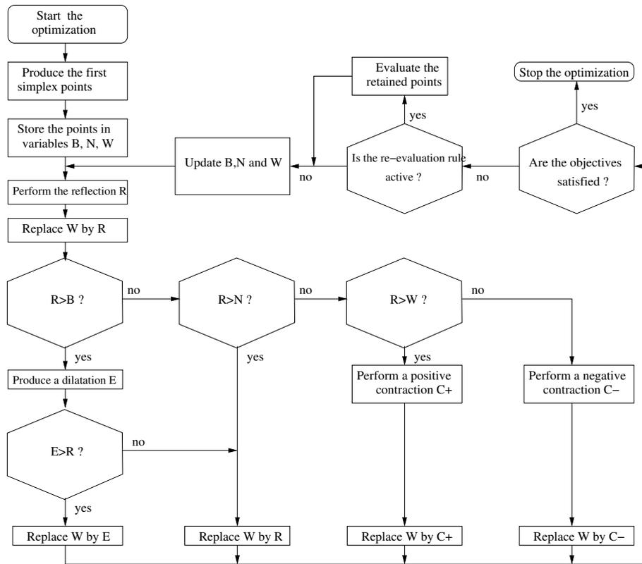
Figure 14.9. Flow chart of the simplex method algorithm.
