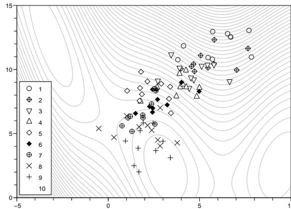
**Figure 14.6.** Example of a `muLambda` optimizer (evolution strategy  $(\mu/\mu, \lambda)$ ) convergence on the Branin-Hoo function with  $\mu = 2$  parents,  $\lambda = 10$  offsprings and 10 iterations (i.e., 100 evaluations in total).
