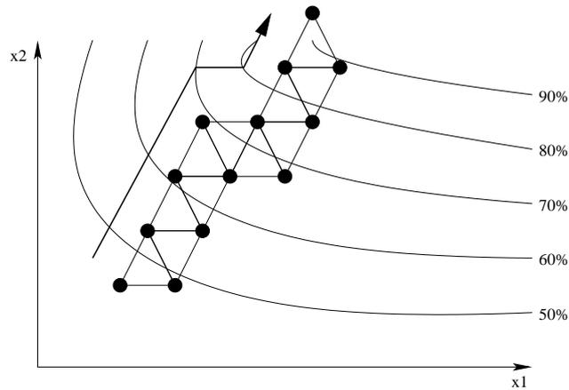
**Figure 14.10.** Path of a simplified simplex method (only reflections are made). The algorithm correctly finds an uphill direction (the function is maximized here).
