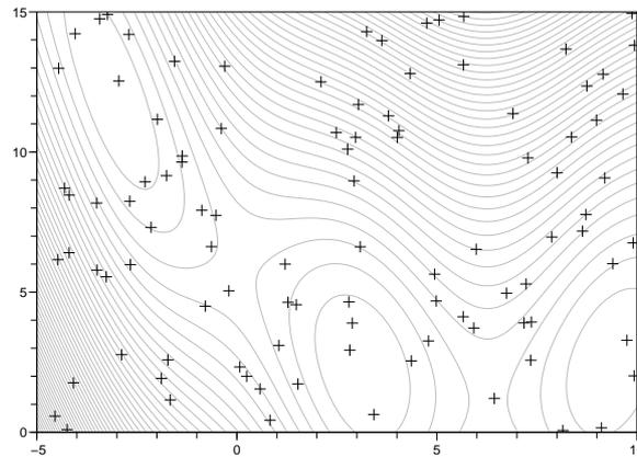
**Figure 14.5.** Sample run of the *rsearch* optimizer with 100 iterations on the Branin-Hoo function.
