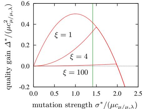
Figure 9: Normalized quality gain of  $(\mu/\mu, \lambda)$ -ES on cigar functions for  $n \rightarrow \infty$  plotted against the normalized mutation strength for  $\xi \in \{1, 4, 100\}$ . The vertical line represents the average normalized mutation strength generated by cumulative step-size adaptation.
