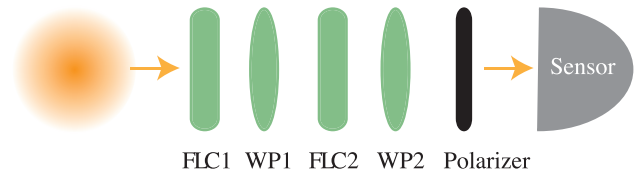
Figure 1: An example 2-FLC polarimeter where the polarization state of incident light is analyzed by the Polarization State Analyzer and a light intensity detector.
