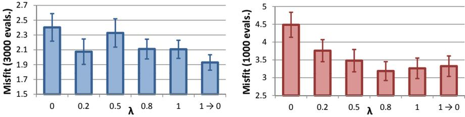
**Fig. 4.** GuPSO performance for different values of  $\lambda$  after 3000 and 1000 solution evaluations, averaged over 30 runs. Standard PSO is provided by setting  $\lambda$  to 0, while the last bar gives the results obtained by allowing  $\lambda$  to vary from 1 (guide objectives only) to 0 (true objective only) linearly over the course of the search.
