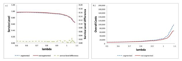
Figure 3: Service level and overall costs for the two machine allocation policies in the four-items-high-lotsize-scenario S1
