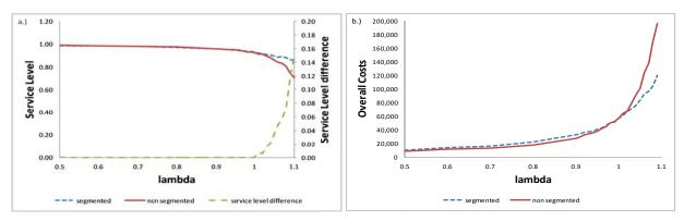
Figure 4: Service level and overall costs for the two machine allocation policies in the four-items-low-lotsize-scenario S2
