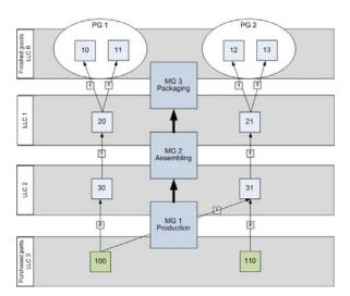
Figure 1: Bill of material and processing structure
