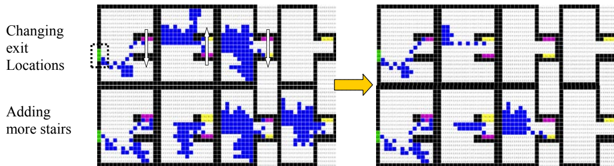
Figure 9: Simulation results of two modified building (exit location changed / more doors added).
