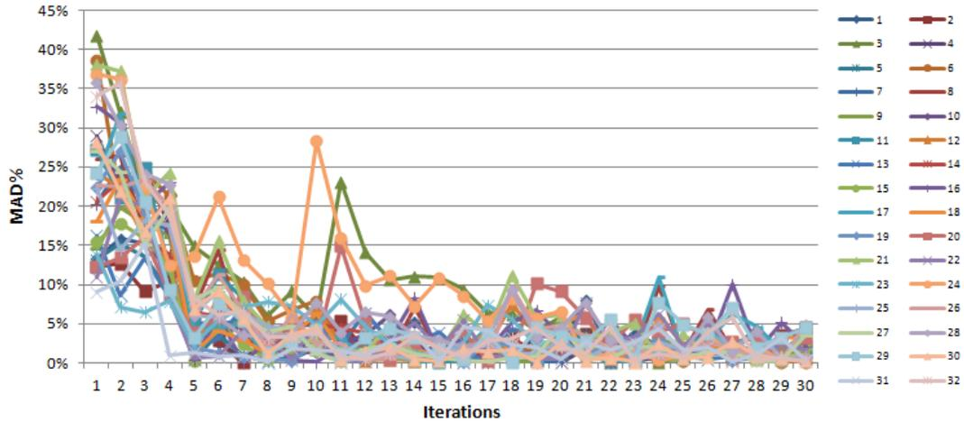
Figure 2: MAD in product cycle times for the (DL=High, ILT=Accurate,  $\alpha=0.20$ ) case.
