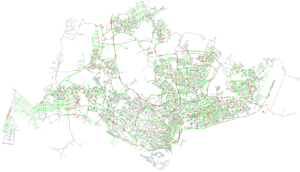
Figure 4: Example of simulation results that indicate the estimated average speed on the various road links of the Singapore road network. The colors green and red indicate that the average speed is expected to be faster or slower, respectively.
