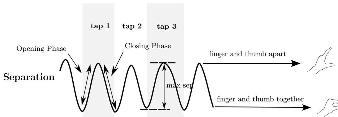
Figure 1: Obtaining the tap separation values.
