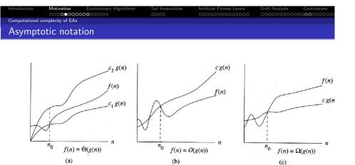
$\begin{array}{ll} f(n) \in O(g(n)) \iff \exists \quad \text{constants} \quad c, n_0 > 0 \quad \text{st.} \quad 0 \leq f(n) \leq cg(n) \quad \forall n \geq n_0 \\ f(n) \in \Omega(g(n)) \iff \exists \quad \text{constants} \quad c, n_0 > 0 \quad \text{st.} \quad 0 \leq cg(n) \leq f(n) \quad \forall n \geq n_0 \\ f(n) \in \Theta(g(n)) \iff f(n) \in O(g(n)) \quad \text{and} \quad f(n) \in \Omega(g(n)) \\ f(n) \in o(g(n)) \iff \lim_{n \to \infty} \frac{f(n)}{g(n)} = 0 \end{array}$
