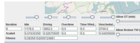
Figure 1: The sliders allow the relative weights to be adjusted during the course of a run depending on the criteria defined by the customer. The Customer can also specify the amount of allowed overtime and the maximum period by which time windows can be broken
