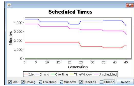
Figure 4: The plot shows the actual times for idle time, driving time, overtime, broken time windows and unscheduled jobs. The display can be switched to show the normalised weighted fitness used to drive evolution.
