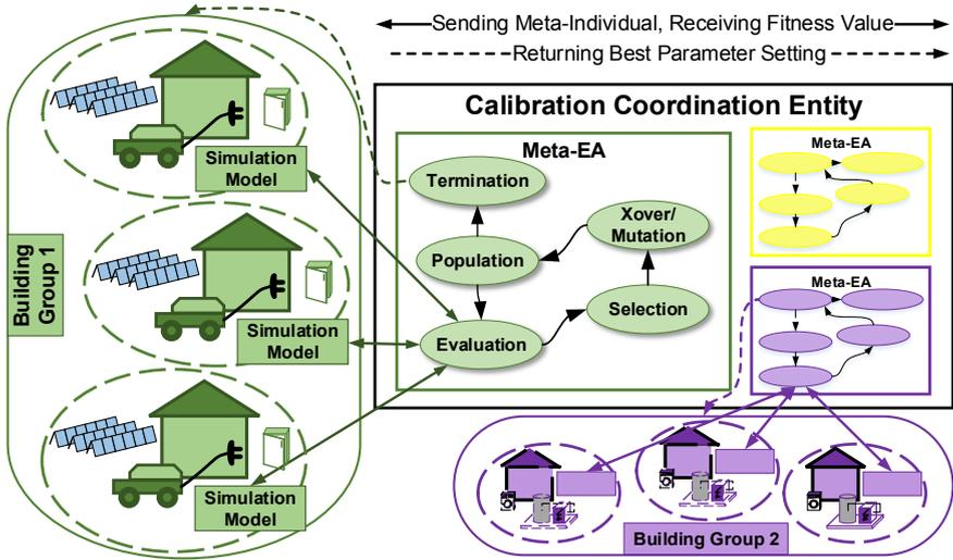
Fig. 4. Calibration Coordination Entity with different groups of buildings
