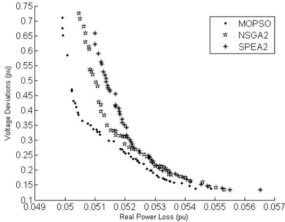
Fig. 1. The best obtained Pareto-fronts of MOPSO, NSGA-II and SPEA2 for the base load of the IEEE30-bus system
