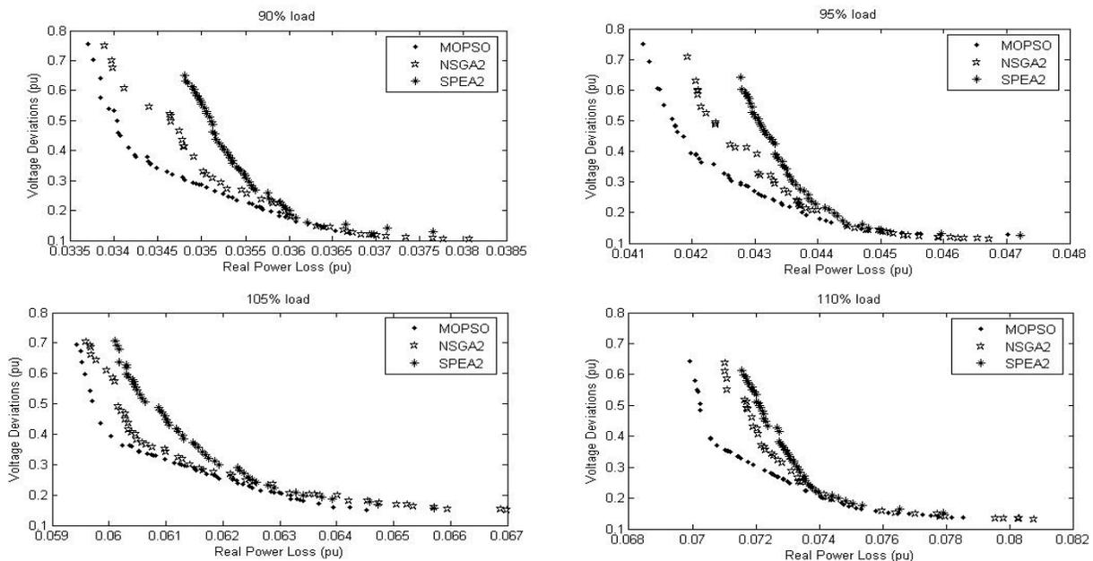
Fig. 2. The best obtained Pareto-fronts of MOPSO, NSGA-II, and SPEA2 for different loading levels of the IEEE30-bus system
