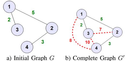
Fig. 4. A complete graph is used by ACO from the initial patrolling graph. Costs of the missing edges are the cumulated distances of the shortest paths.
