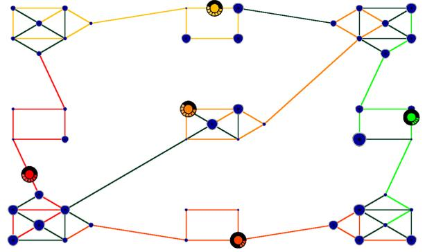
Fig. 1. Snapshot of a multi-agent patrolling strategy involving 5 agents on a 50-node graph. Blue circles represent nodes. Sliced circles are agents. The instantaneous idleness of a node is indicated by the size of its circle. Colored edges link the nodes visited infinitely often by the agents in their cycles. Black edges are not taken by any agent during cycles.
