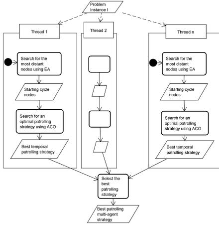
Fig. 6. Flowchart of a Multi-Core ACO/EA Algorithm
