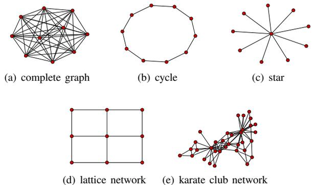
Fig. 1. Some representative network structures. The top row shows the structures of complete graph, cycle and star with the network size  $N = 10$ . The bottom row depicts the structures of lattice network and the karate club network. The size of the lattice network is  $N = 9$ , and the karate club network is a connected and undirected network with 34 nodes and 78 edges.
