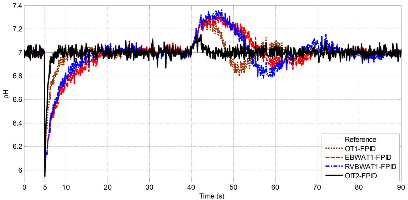
Fig. 9. Illustration of the input and output disturbances rejection performances of the fuzzy PID control systems
