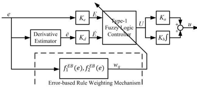
Fig. 4. Illustration of the EBWAT1-FPID controller structure
