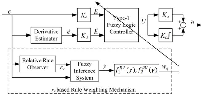
Fig. 6. Illustration of the RVBWAT1-FPID controller structure
