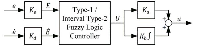
Fig. 2. Illustration of the T1-FPID / IT2-FPID controller structure
