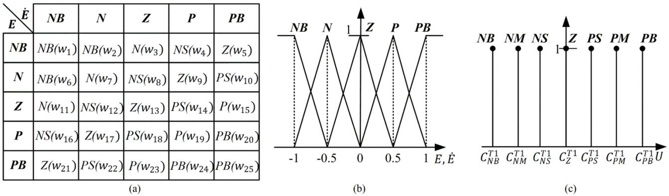
Fig. 3. Illustration of the (a) Rule base of T1-FLC, (b) Antecedent MFs of T1-FLC, (c) Consequent MFs of T1-FLC
