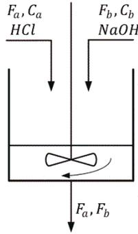
Fig. 1. Illustration of pH neutralization process
