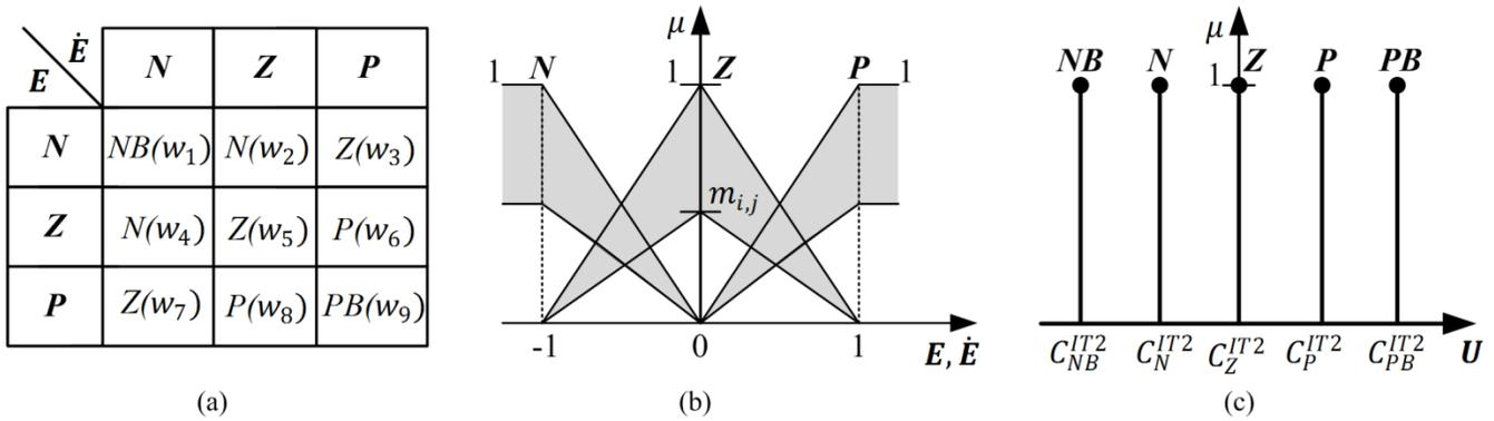
Fig. 7. Illustration of the (a) Rule base of IT2-FLC (b) Antecedent MFs of IT2-FLC, (c) Consequent MFs of IT2-FLC
