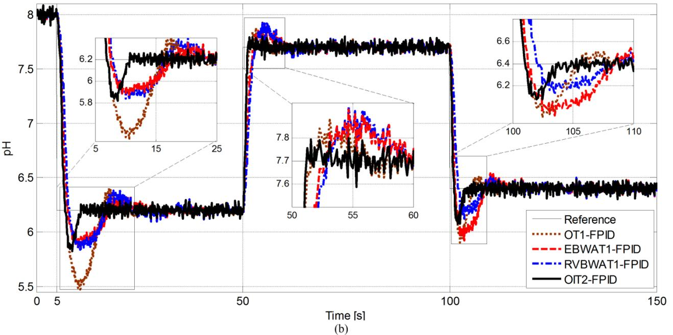
Fig. 8. Illustration of the responses of the fuzzy PID control systems for the (a) control performance studies, (b) the robustness performance studies
