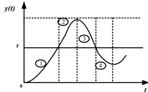
Fig. 5. Illustration of the partitioning of the step response
