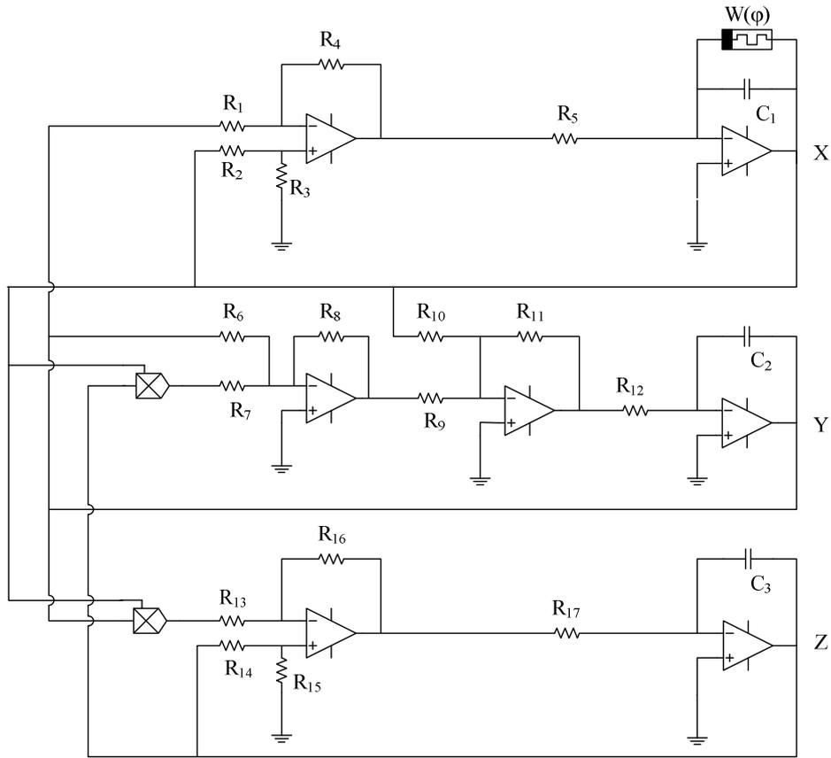
Fig. 2. Memristor-based Lorenz circuit.
