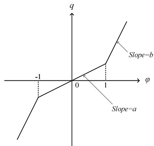
Fig. 1. The constitutive relation of the flux-controlled memristor.
