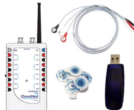
Fig. 3. EMG electrodes with wireless BioRadio and USB receiver from ClevMed. Inc.
