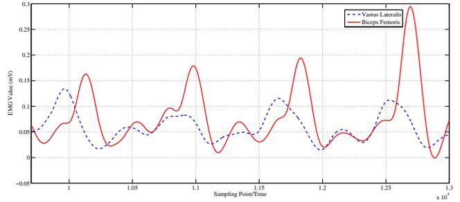
Fig. 5. Characteristics for vastus lateralis (---) and biceps femoris (—) muscles in the ACL-R leg of a subject 1 year after surgery during walking for multiple gait cycles
