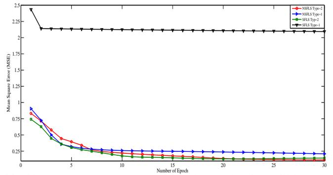
Fig. 15. Average mean square error (MSE) for type-1 and type-2 FL systems for during training phase
