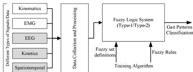
Fig. 1. General framework for classification of gait patterns of ACL-R subjects using adaptive fuzzy logic system
