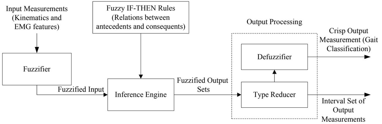
Fig. 7. Type-2 fuzzy logic based framework to build the gait patterns' classification model
