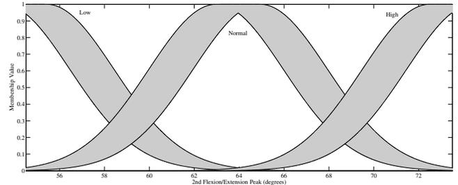
Fig. 11. Type-2 Gaussian membership functions for 2nd flexion/extension peak during a gait cycle
