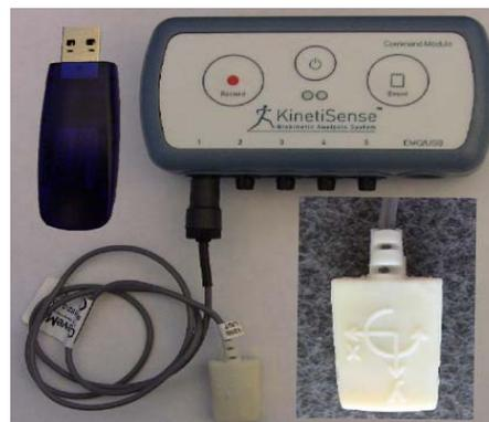
Fig. 2. Wireless motion sensor unit command module and USB receiver from KinetiSense (ClevMed. Inc.)
