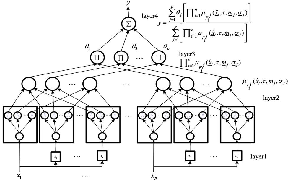
Fig.1 The adaptive time delay FNN structure.
