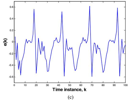
Fig. 3. (a) The testing input  $u(k) = \sin(2\pi k / 25)$ . (b) The output of the T-S affine linear model (dotted line) and the plant (solid line). (c) Errors between the outputs of fuzzy bilinear model and plant for test input with  $L = 100$  (MSE = 0.0689).
