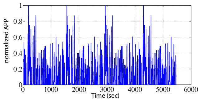
(c) Normalized accelerator pedal position
