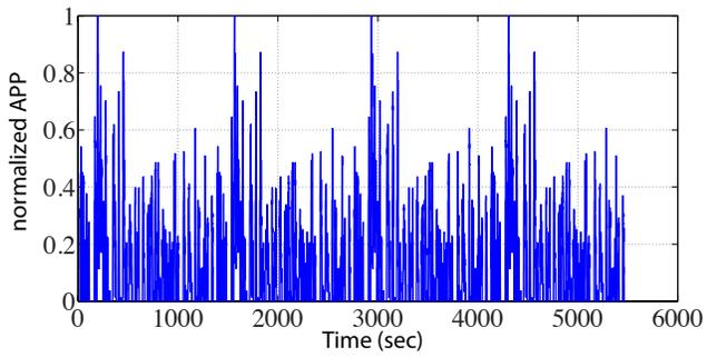
(c) Normalized accelerator pedal position
