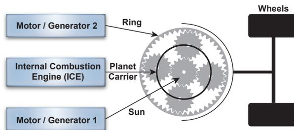
Fig. 1. HEV power split transmission block diagram
