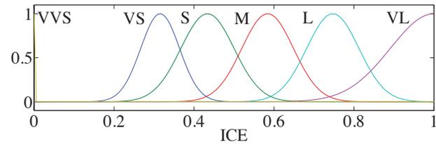
Fig. 6. MFs for Normalized ICE Torque Req
