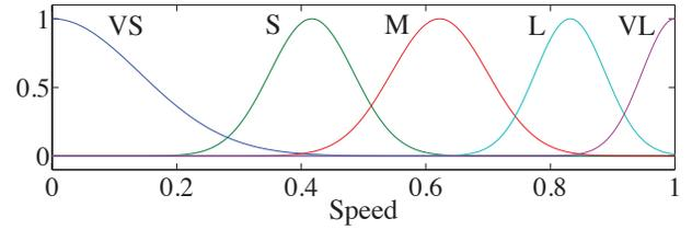
Fig. 2. MFs for normalized vehicle speed
