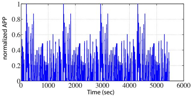
(c) Normalized accelerator pedal position
