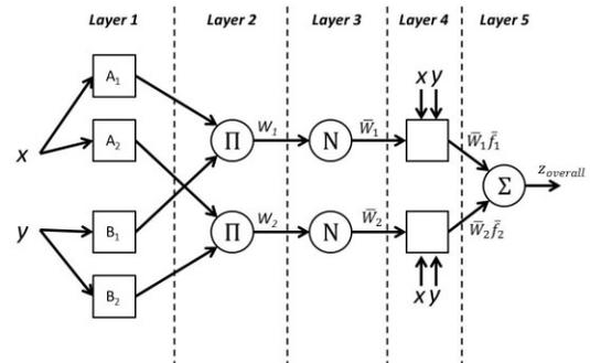
Fig. 6. ANFIS architecture for a two-input first order Sugeno fuzzy model with two rules.
