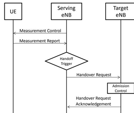
Fig. 2. The figure above shows the summary of the handover procedure in LTE. The above is one part of the three phases the handover procedures of LTE; the handover preparation phase. The subsequent two phases known as the handover execution and handover completion phases, are not the focus of this paper.
