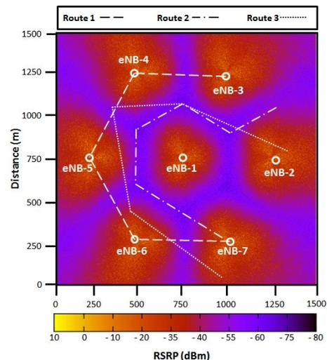
Fig. 10. The radio environment map which consists of seven eNB generated to simulate the scenarios.
