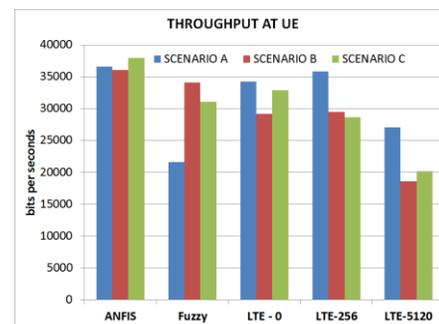
Fig. 14. The comparison of handover algorithms for UE downlink throughput.
