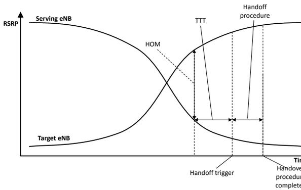
Fig. 3. The handover trigger algorithm for LTE. In order to trigger the handover procedure, the target eNB RSRP must be higher than the HOM for a period of TTT.
