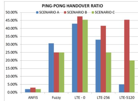
Fig. 12. The graph of comparison of ANFIS, fuzzy and LTE handover decision algorithms for the ping-pong handover ratio,  $H_{PHR}$ . LTE handover algorithm is compared with TTT=0ms (LTE-0), TTT = 266ms and TTT= 5120ms (LTE-5120) respectively.
