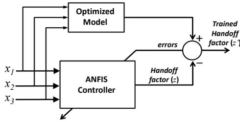
Fig. 8. ANFIS training for the proposed LTE handover trigger algorithm.  $x_1$ ,  $x_2$  and  $x_3$  can be represented as RSRP, BLER and QoS parameters depending on the local requirements of the UE and service provider.
