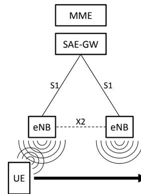
Fig. 1. The LTE network architecture based on S1 and X2 handover protocol. Each eNB is connected to System Architecture Evolution Gateway (SAE-GW) which houses the mobility management entity (MME).
