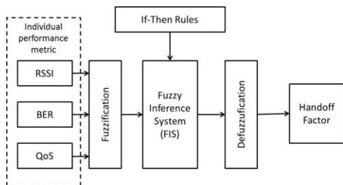
Fig. 4. The block diagram of a fuzzy logic handover decision algorithm. At the output of the defuzzification process, a string of data known as the handoff factors are generated.
