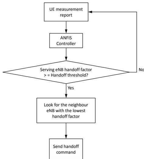
Fig. 9. Flowchart of the LTE handover trigger phase.
