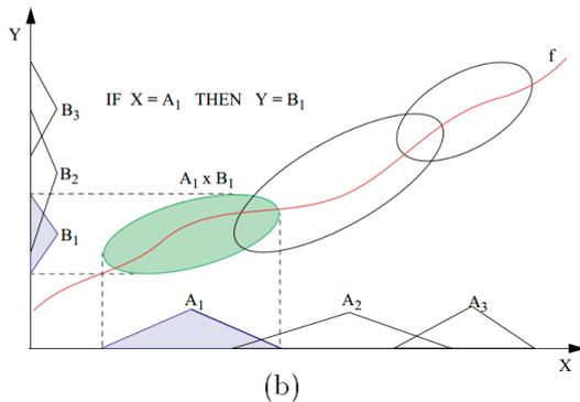
Fig. 2. (a) A configuration of SAM. Each input fires each fuzzy rule to some degree to calculate  $F(x)$ . (b) Fuzzy rules specify patches in the input-output space [15].
