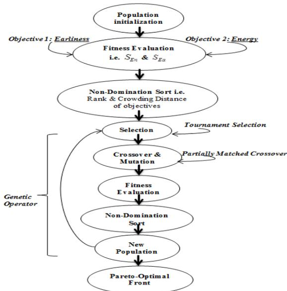
Fig. 4: Flow-Chart of Modified NSGA-II
