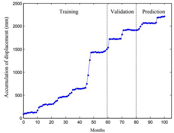
Fig. 1. Monitoring curves of landslide accumulative displacement at ZG118 point
