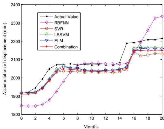
Fig. 2. The comparison between monitoring data and prediction results
