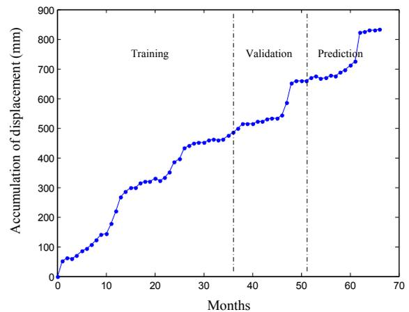
Fig. 3. Monitoring curves of landslide accumulative displacement at Z111 point
